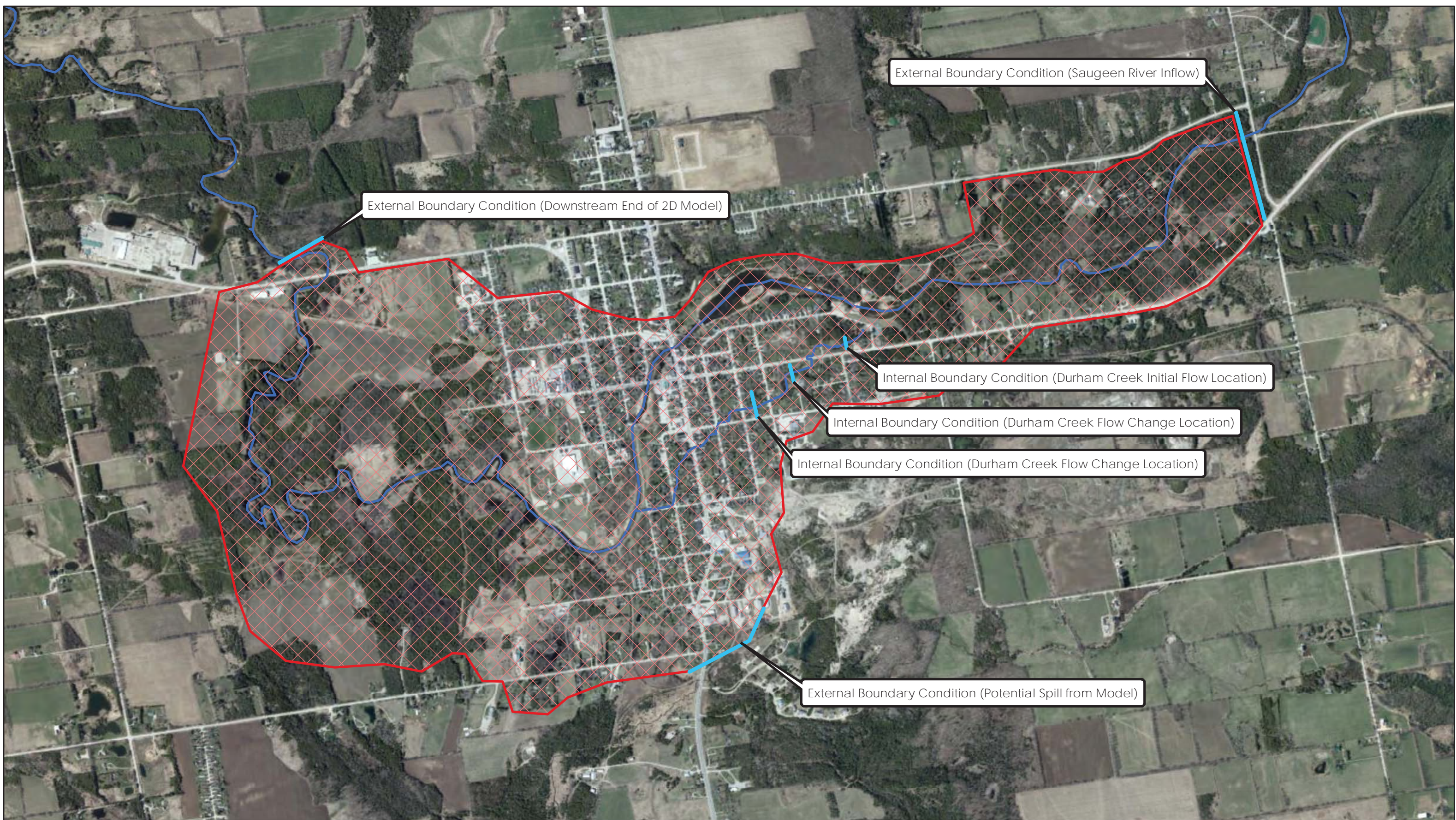
Figure 12 Saugeen River and Durham Creek Hydraulic Modelling Domain
